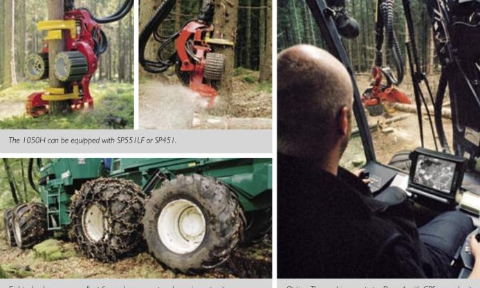
Eight wheels ensure excellent forward movement and carrying capacity. The bogielift at the rear can be used, for instance, for fast entering thinning areas.
