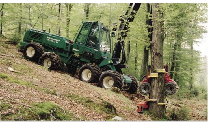
The stability in longitudinal direction permits working on steep slopes even with full reach of the boom. The operator's work environment is comfortable und ergonomic with low noise level, pleasant air condition and thanks to the large windows and the narrow pillars excellent visibility throughout the working area.
