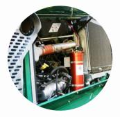
The engine is a step V without EGR valve. The after-treatment of the exhaust gases is done in a Single Module. It takes up less space, resulting in significantly decreased installation dimensions.
